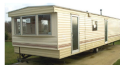
Mobile Home - factory built, remains on a steel chassis & built pre-1976 - no HUD Code
